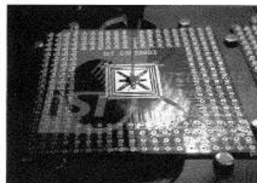
圖4 點膠(Adhesive Dispensing)
