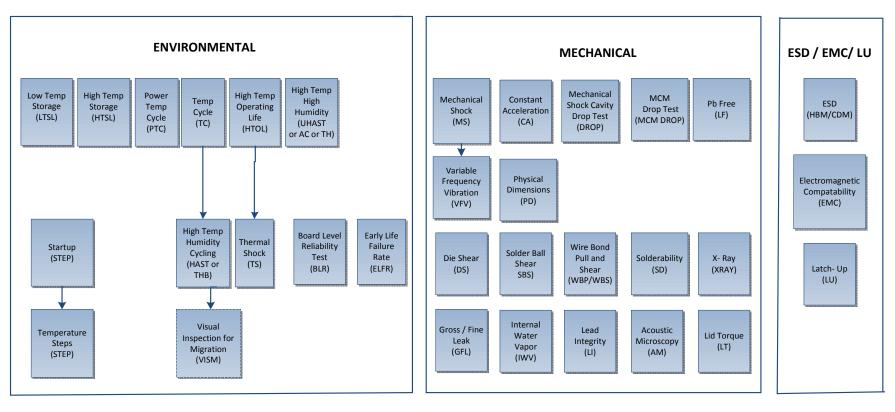
Note: Pre-conditioning (PC) to simulate customer manufacturing and rework processes is required for the package accelerated environmental stress tests (test group A). See Tables 1 & 2 for applicability of each test.
